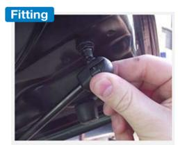
Push the ball socket over the ball stud - you will feel it click into place. If the sockets do not line up with the ball studs then grip the cylinder by hand and rotate it clockwise.
