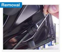
Slide a flat blade screwdriver under the metal band. Lever the band back and pull on the gas strut to remove it from the vehicle. You do not need to remove the band to do this.
