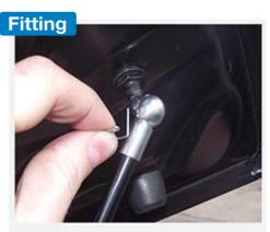
To fit your new gas struts remove the pin, push fit onto the ball stud & replace the pin. If the sockets do not line up with the ball studs then grip the cylinder and rotate it clockwise.
