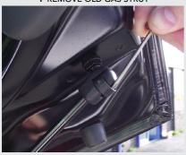
Slide a flat blade screwdriver under the metal band. Lever the band back and pull on the gas strut to remove it from the vehicle. You do not need to remove the band to do this.
