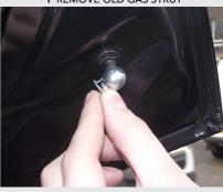
Unclip the small pin from around the base of the ball and totally remove it from the fitting. Once the pin is separate the gas strut can be removed, leaving just the ball attached.
