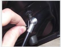
To fit your new gas struts remove the pin, push fit onto the ball stud & replace the pin. If the sockets do not line up with the ball studs then grip the cylinder and rotate it clockwise.
